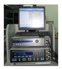
The Solartron Analytical 1287 coupled with frequency response analyzer 1260 as an electrochemical workstation can offer high accuracy, wide band, potentiostat/galvanostat testing service.
