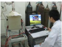
SOFCMAN has 8 sets of 100W single cell testing equipments, 2 set of button cell testing equipments and a set of electrochemical workstation the Solartron Analytical 1287 coupled with frequency response analyzer 1260. We offer SOFC cell testing service including I-V measurement, cell resistance testing, AC impedance testing and duration test of single cells.
